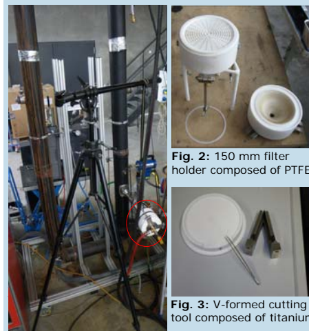
Fig. 1: Dilution tunnel with the affixed 150 mm filter holder.
