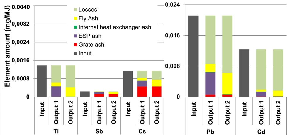
Fig. 4: Amount of heavy metals in wood (source), different ash fractions (sinks) and calculated losses during the production of 1 megajoule (MJ) net energy from burning spruce wood chips; Boiler: Guntamatic Powerchip 20/30, 30 kW, with and without an electrostatic precipitator (ESP)
