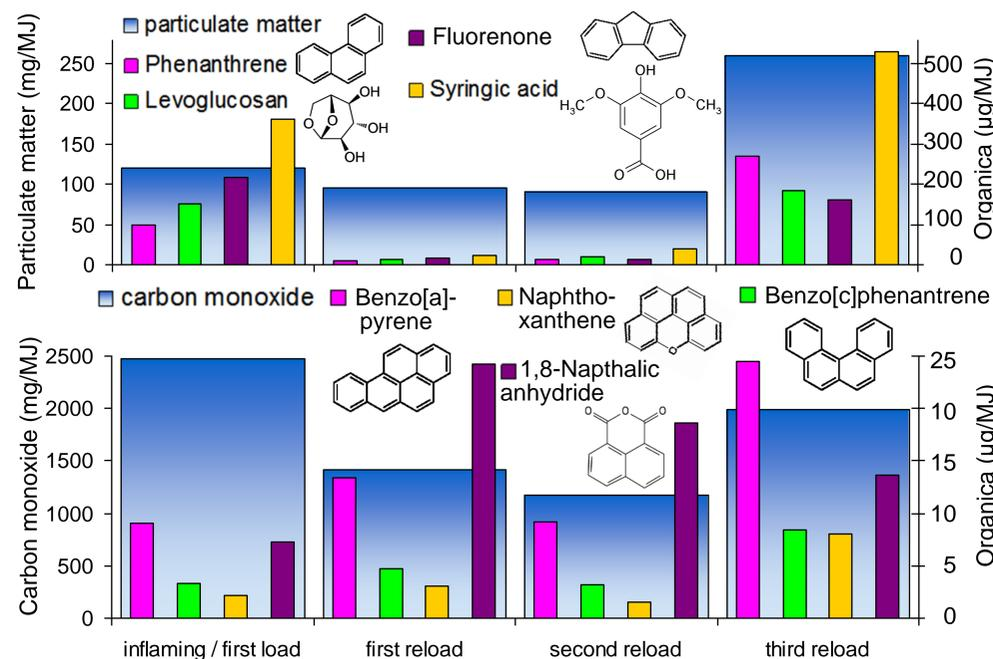
Fig. 5: Emission profile of a wood log stove during different stages of burning. The third reload comprises a 10 minutes smouldering phase. Stove: Buderus BlueLine, 8 kW; Fuel: beech wood log. Combustion time for each load: 45 min. Left axis: Particulate Matter and CO, respectively. Right axis: different organic compounds (Levoglucosan: multiply axis by 100).
