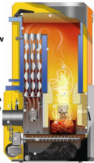
Fig. 1: Furnace Guntamatic Powerchip 20/30
